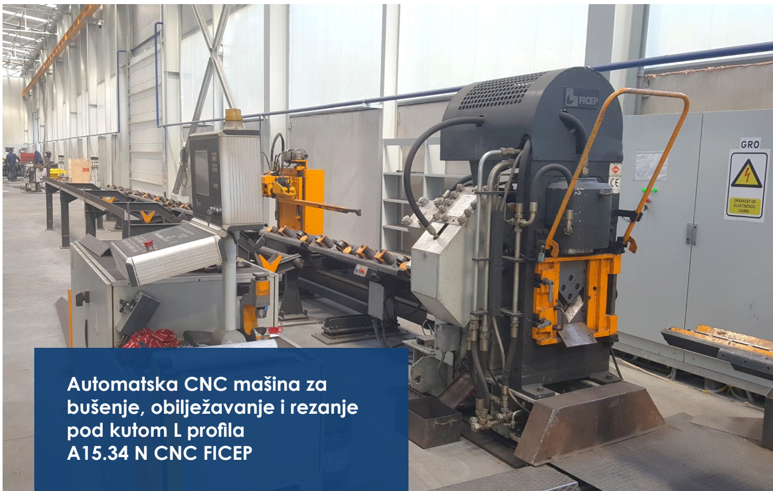
Automatic CNC drilling, marking and cutting at the angle of the L profiles A15.34 N CNC FICEP
